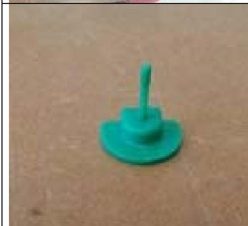
This is the type of plastic safety clip that was missing from Private Ross' life jacket. This plastic pin passes through the firing head body and firing level to act as a resistive force against inadvertent deployment of the jacket as well as a visible indicator that the jacket has not been previously deployed. This clip would normally be ejected from the firing head when the firing lever is pulled.
