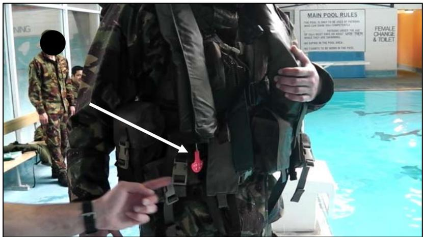
Figure 8: RFB 60B life jacket with toggle exposed
