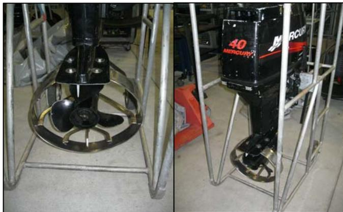
Figure 15: RNZN Outboard Motors with Propeller Guards
