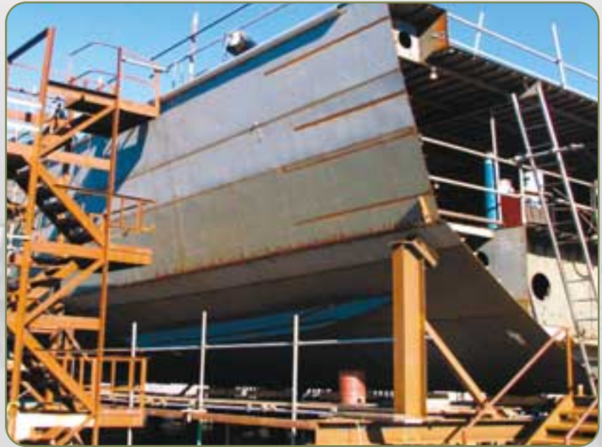
Hull modules of the future Inshore Patrol Vessel Rotoiti consolidated at Tenix NZ yard.
